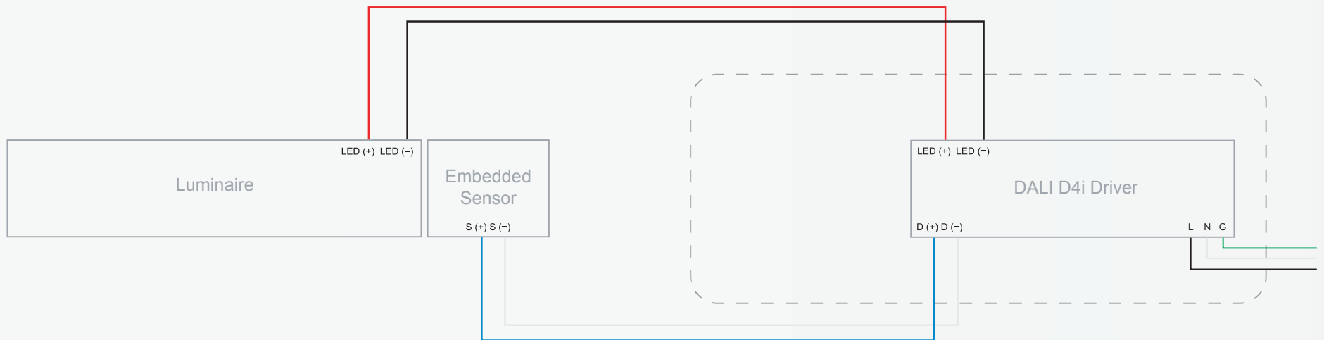
B DALI D4i driver without control unit
