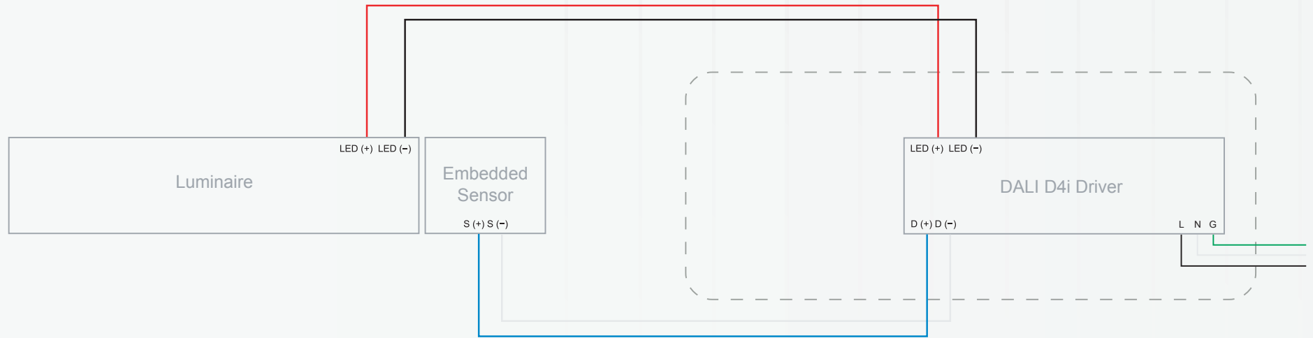
C DALI D4i driver without control unit
