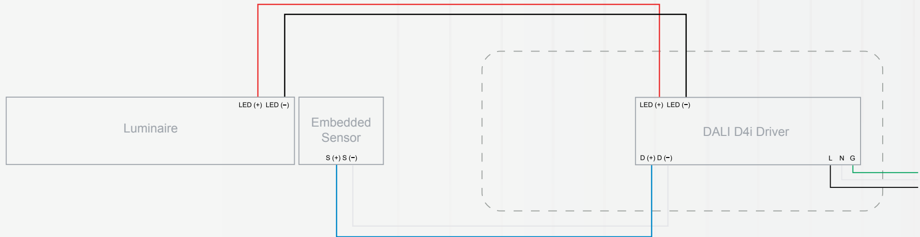
C DALI D4i driver without control unit
