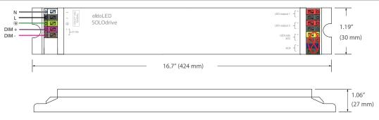
Dimming Control: 0-10v (isolated)
