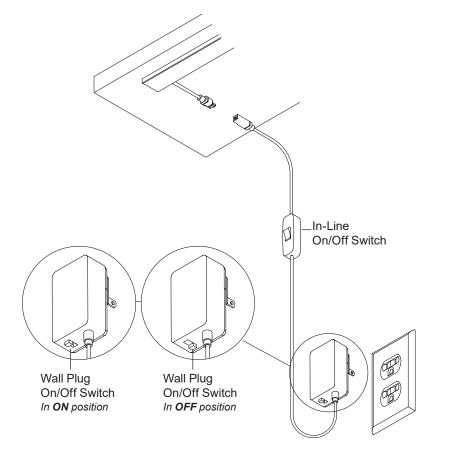
Surface Mount | 707 | ZipOne | Remote Power | Magnet with Tape-On Metal Strip | Installation Guide | August 2020 | Rev A + 4 of 7
