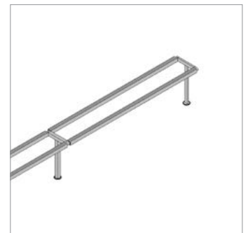
Double Rail with Tee, Arm Anchor
