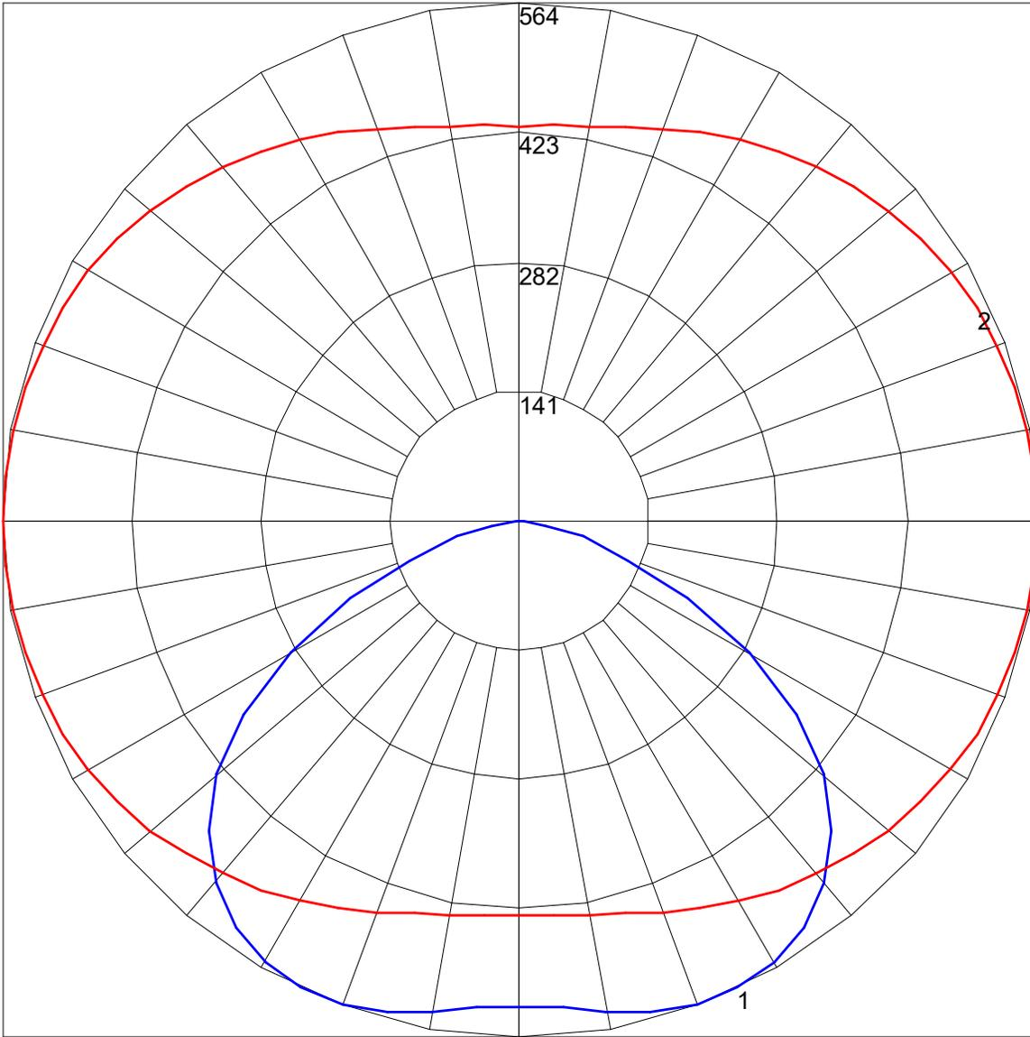
Maximum Candela = 564.311 Located At Horizontal Angle = 0, Vertical Angle = 25
