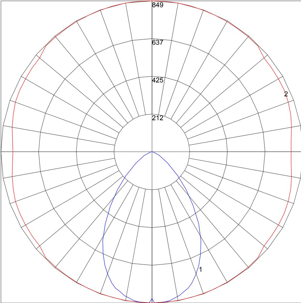
Maximum Candela = 849.05 Located At Horizontal Angle = 90, Vertical Angle = 3
