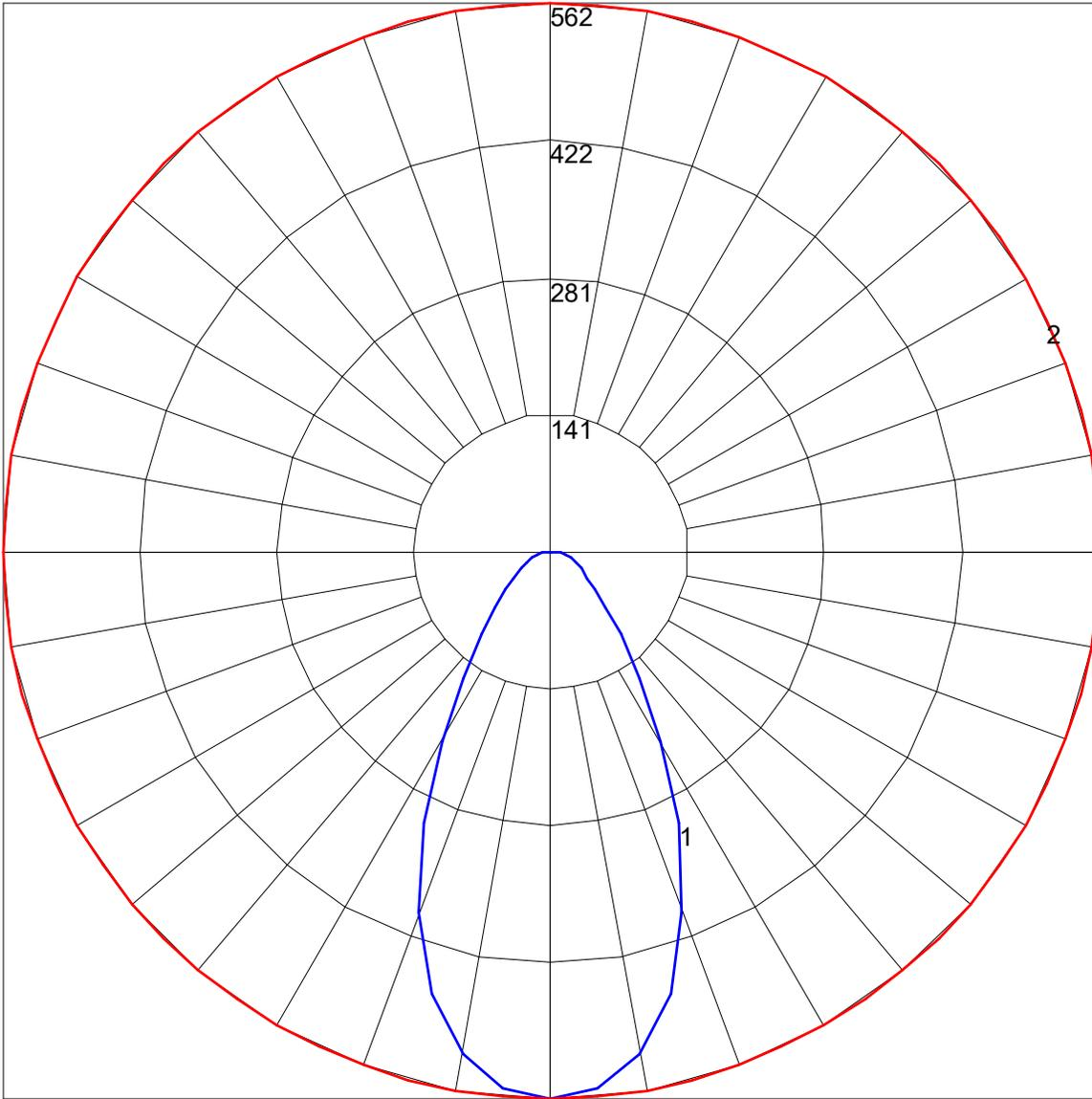
Maximum Candela = 562 Located At Horizontal Angle = 0, Vertical Angle = 0
