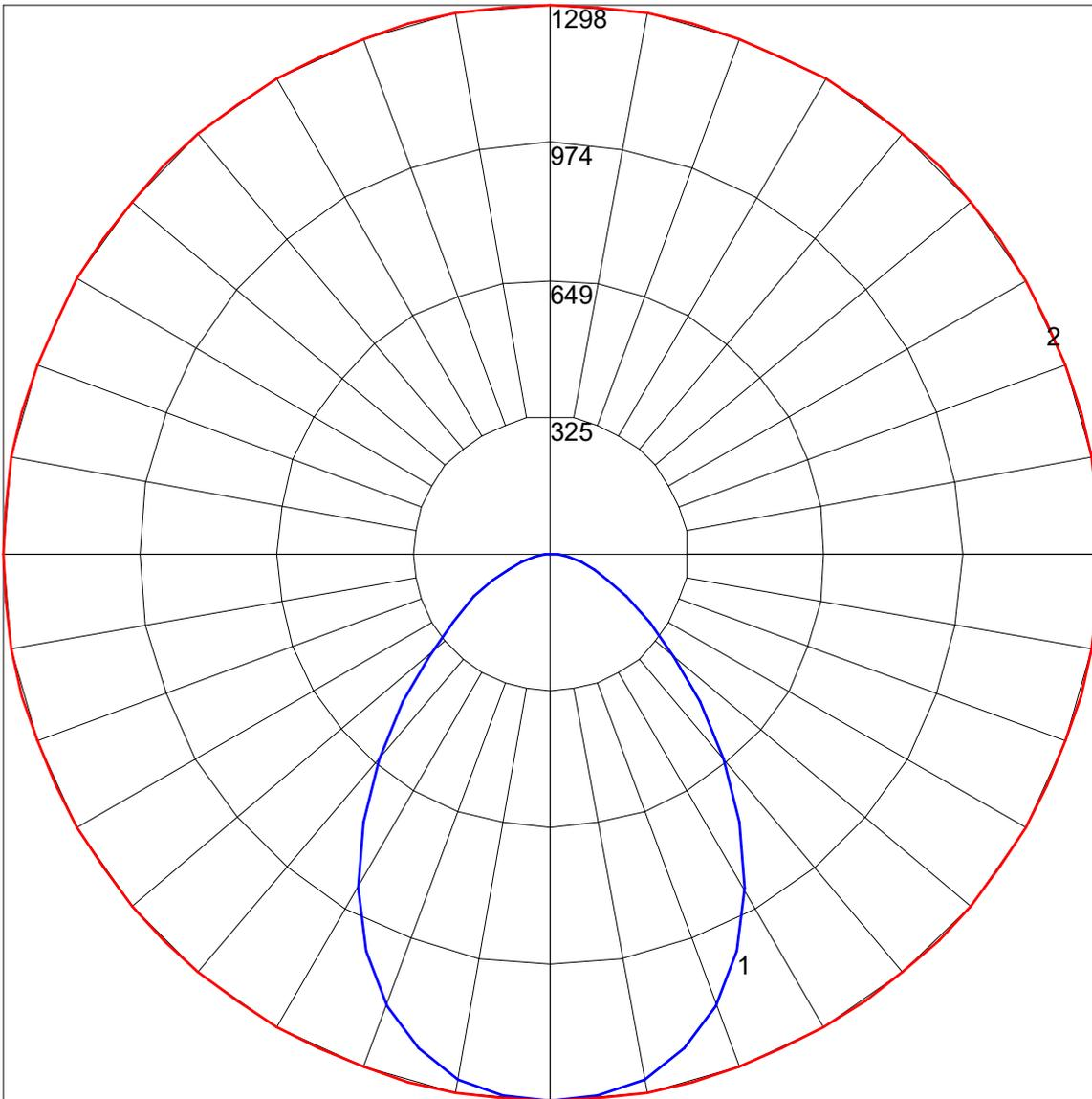
Maximum Candela = 1298.04 Located At Horizontal Angle = 0, Vertical Angle = 0
