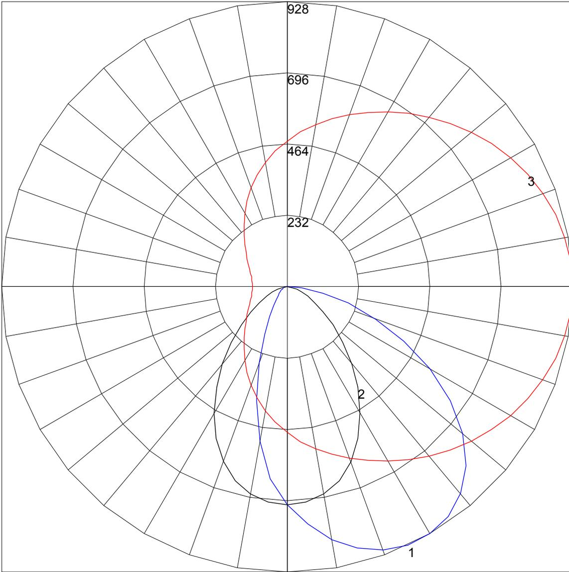
Maximum Candela = 928.44 Located At Horizontal Angle = 0, Vertical Angle = 30
