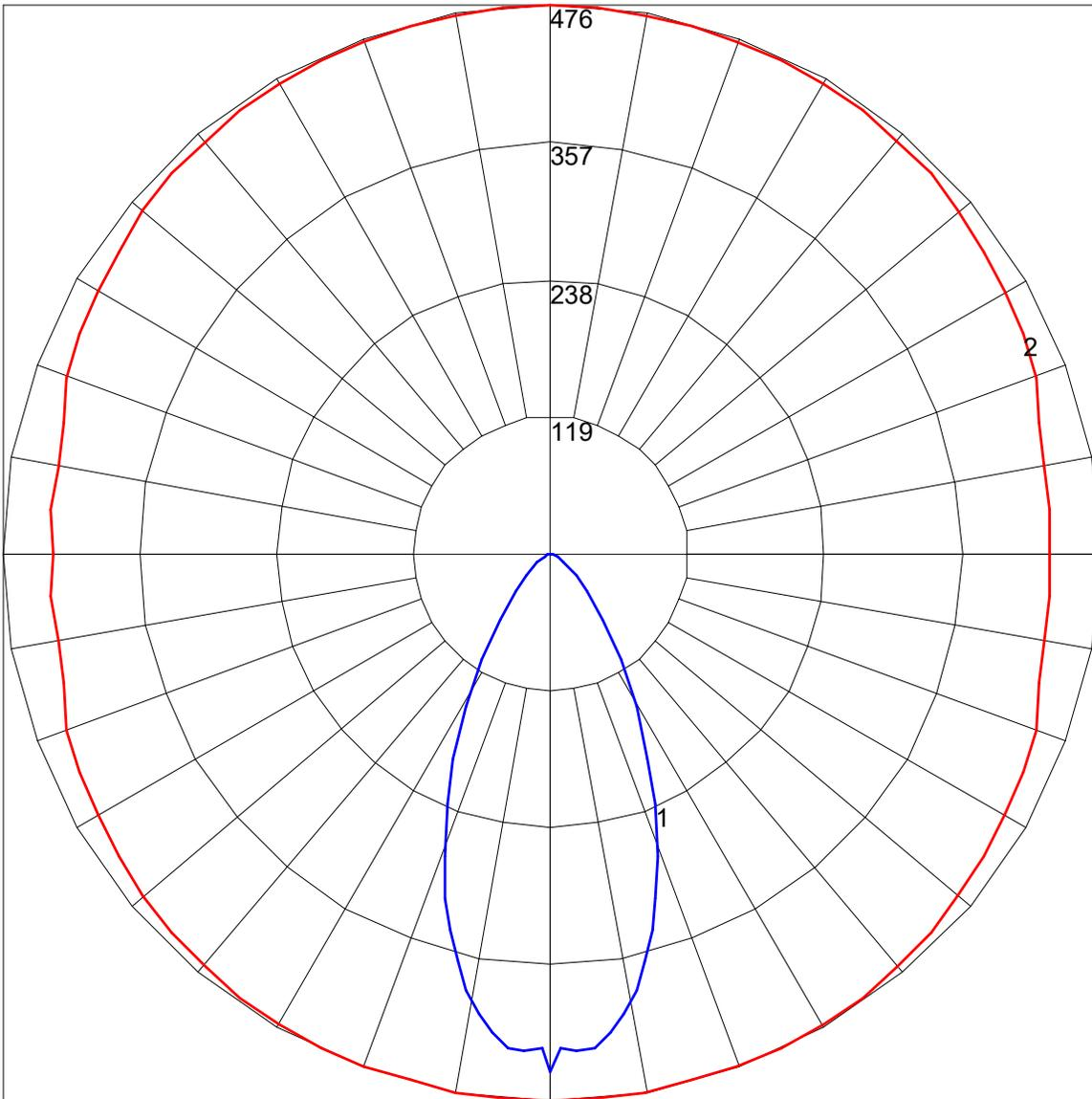
Maximum Candela = 476.415 Located At Horizontal Angle = 90, Vertical Angle = 3
