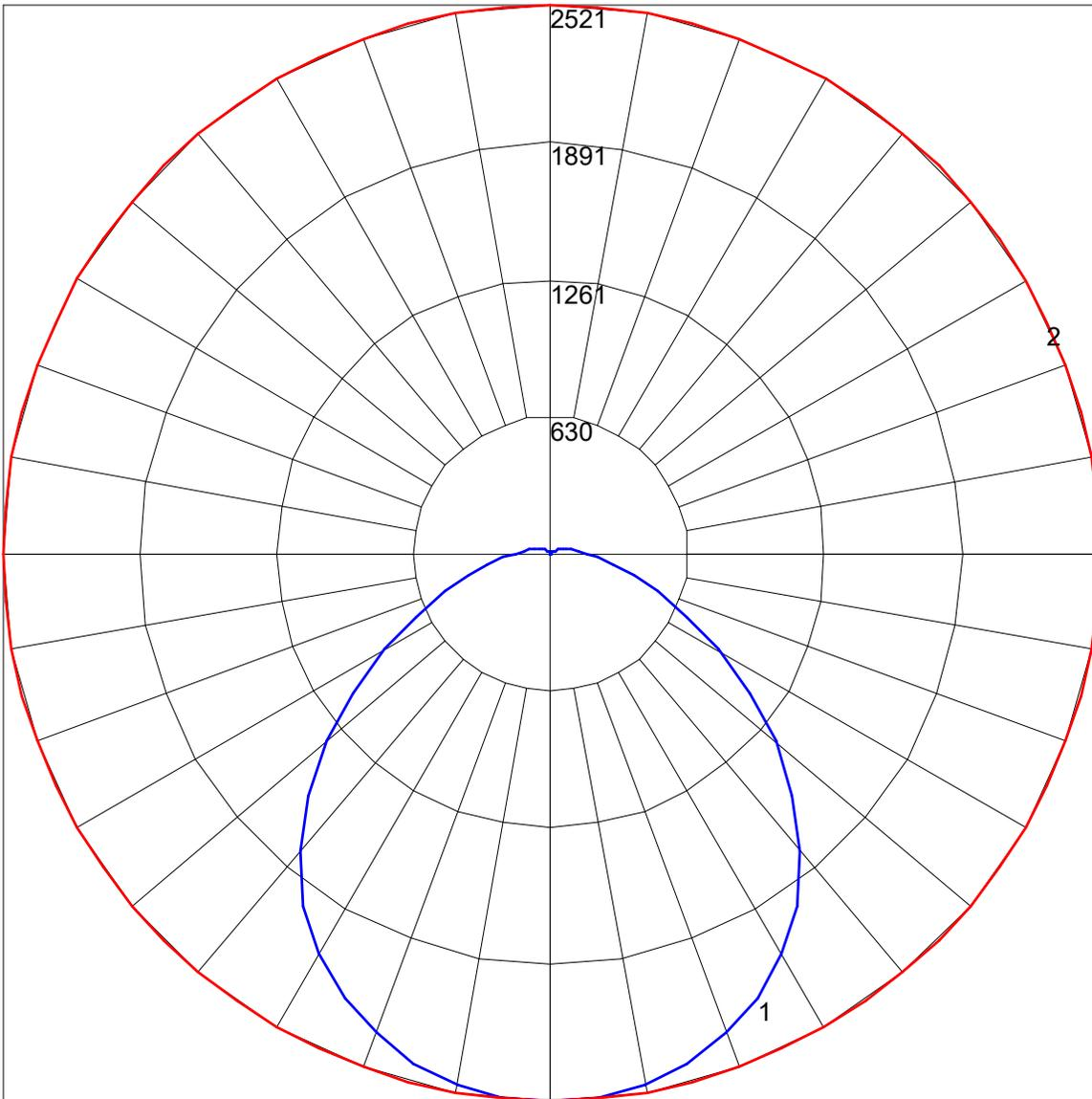
Maximum Candela = 2521.2 Located At Horizontal Angle = 0, Vertical Angle = 0
