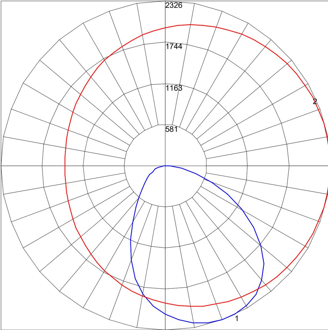
Maximum Candela = 2325.6 Located At Horizontal Angle = 0, Vertical Angle = 20
