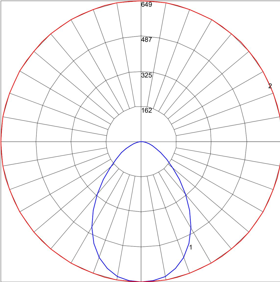
Maximum Candela = 649.02 Located At Horizontal Angle = 0, Vertical Angle = 0
