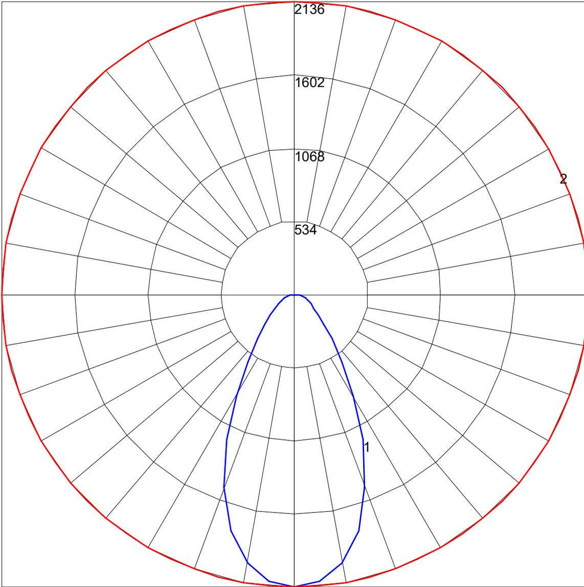
Maximum Candela = 2135.6 Located At Horizontal Angle = 0, Vertical Angle = 0
