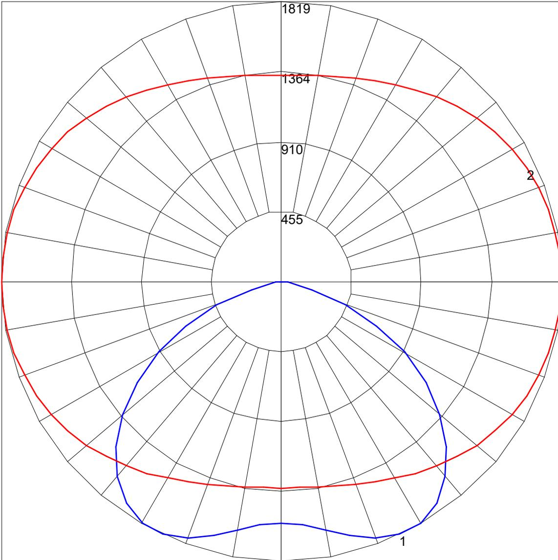
Maximum Candela = 1819.288 Located At Horizontal Angle = 0, Vertical Angle = 25
