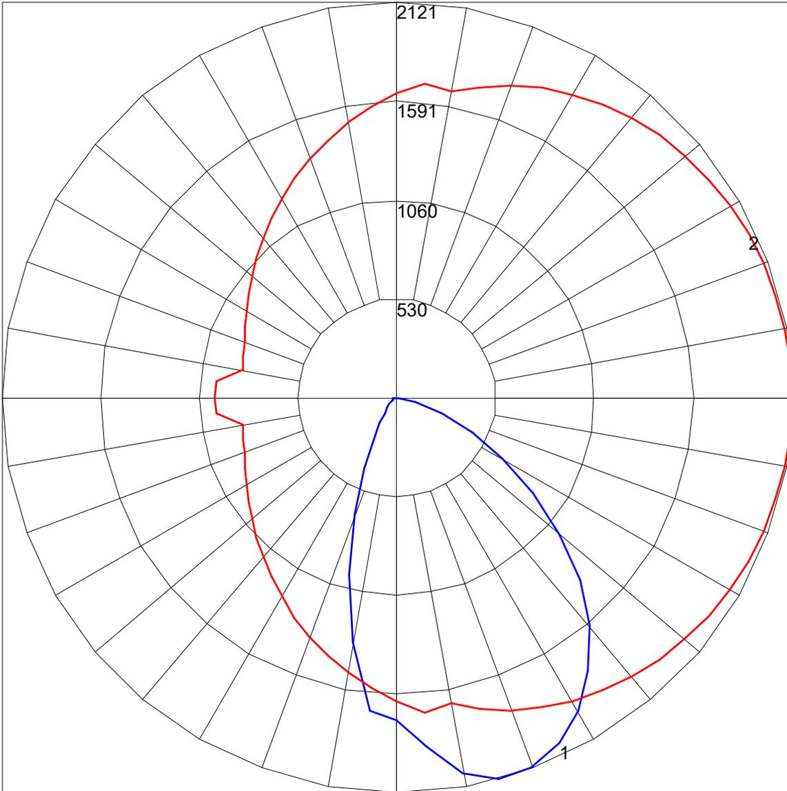
Maximum Candela = 2120.756 Located At Horizontal Angle = 0, Vertical Angle = 15
