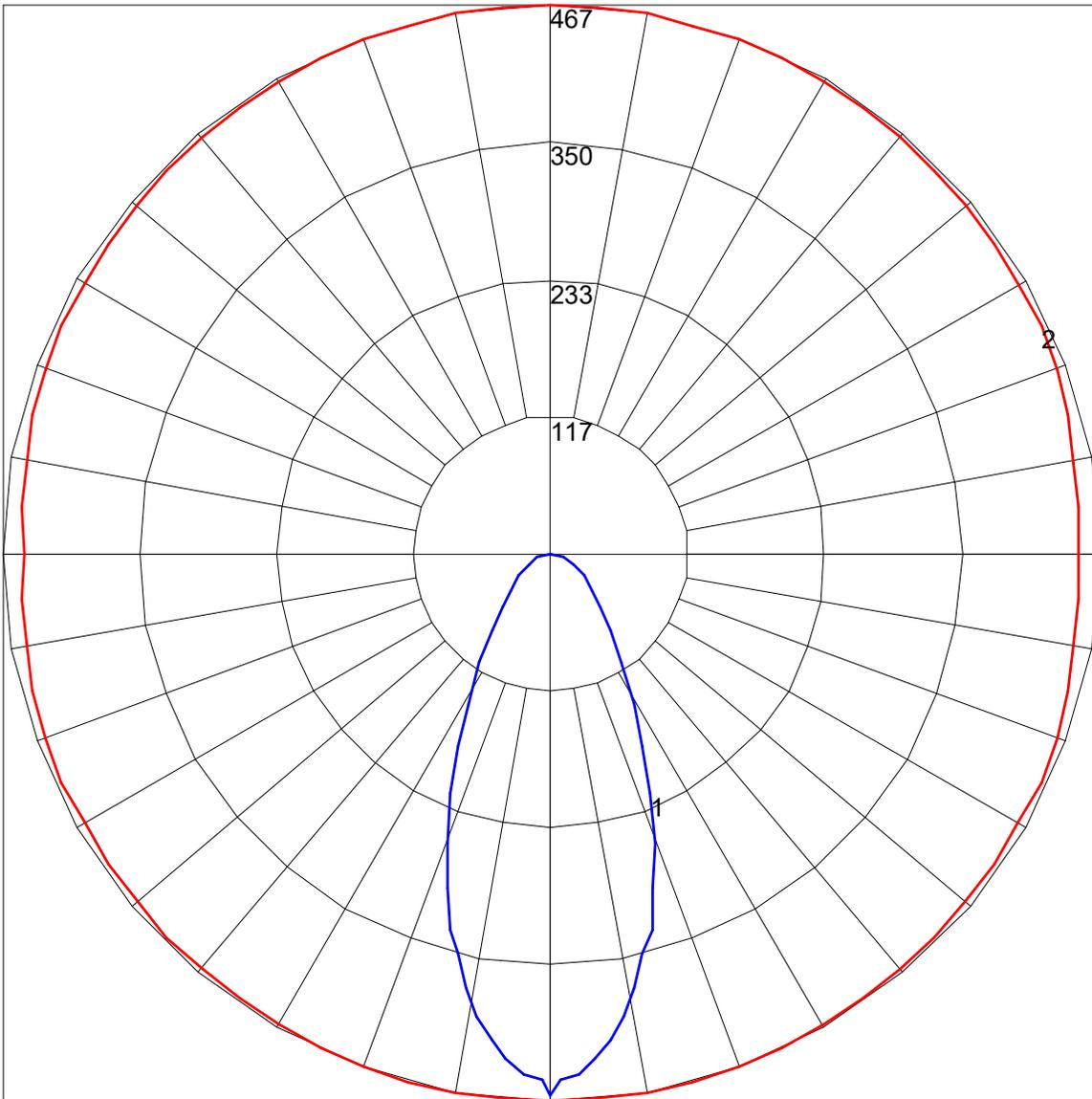
Maximum Candela = 466.73 Located At Horizontal Angle = 80, Vertical Angle = 1
