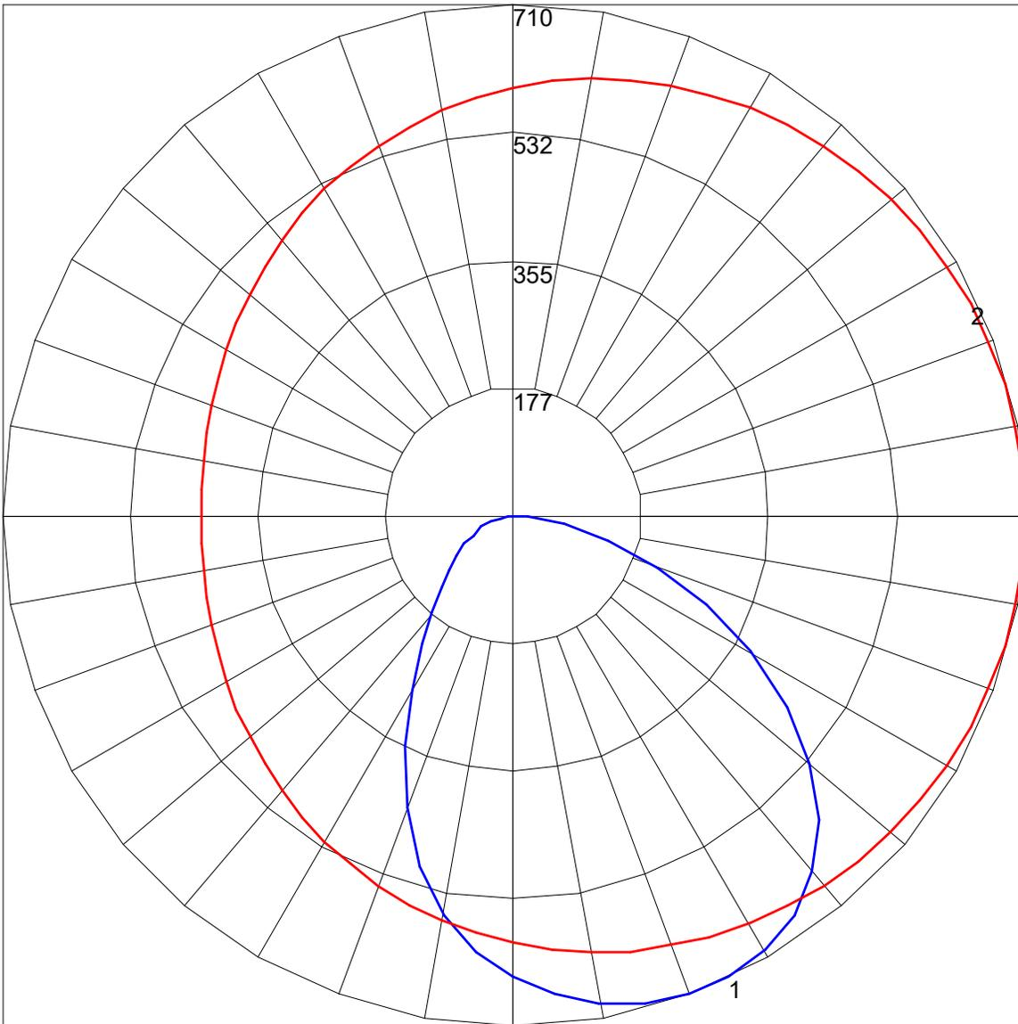
Maximum Candela = 709.92 Located At Horizontal Angle = 0, Vertical Angle = 20
