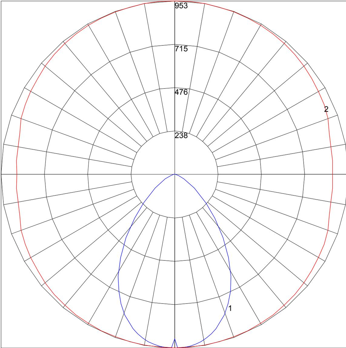
Maximum Candela = 952.83 Located At Horizontal Angle = 90, Vertical Angle = 3
