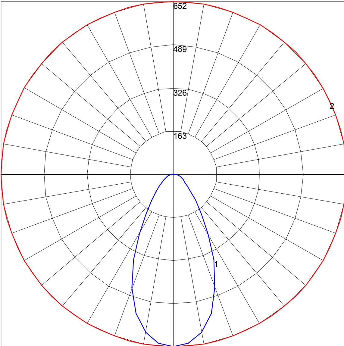
Maximum Candela = 651.92 Located At Horizontal Angle = 0, Vertical Angle = 0
