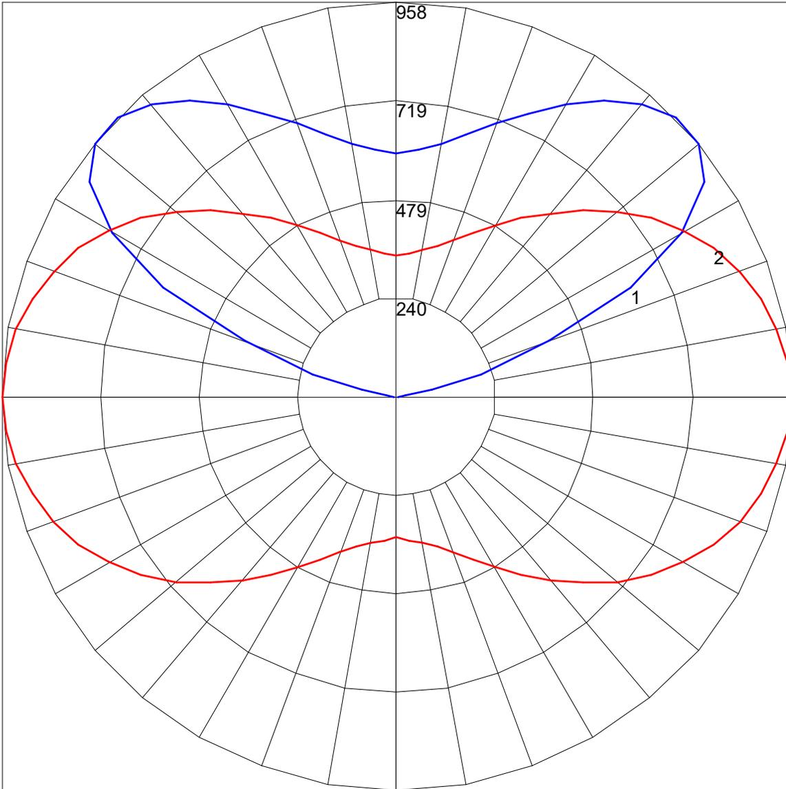
Maximum Candela = 958.45 Located At Horizontal Angle = 0, Vertical Angle = 130
