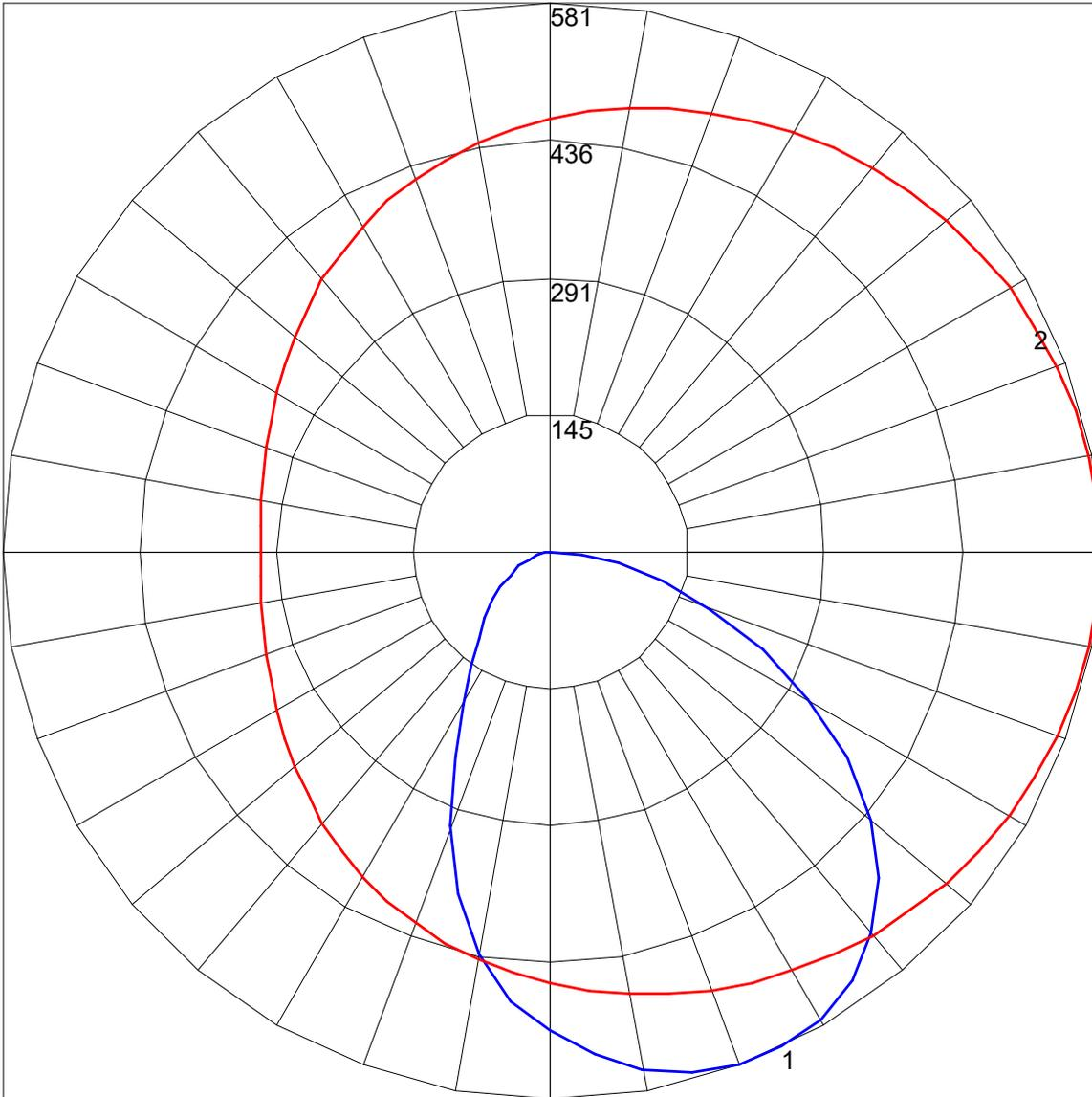
Maximum Candela = 581 Located At Horizontal Angle = 0, Vertical Angle = 20
