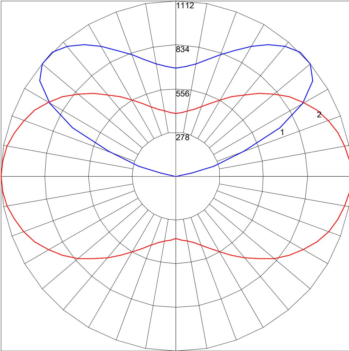
Maximum Candela = 1111.802 Located At Horizontal Angle = 0, Vertical Angle = 130
