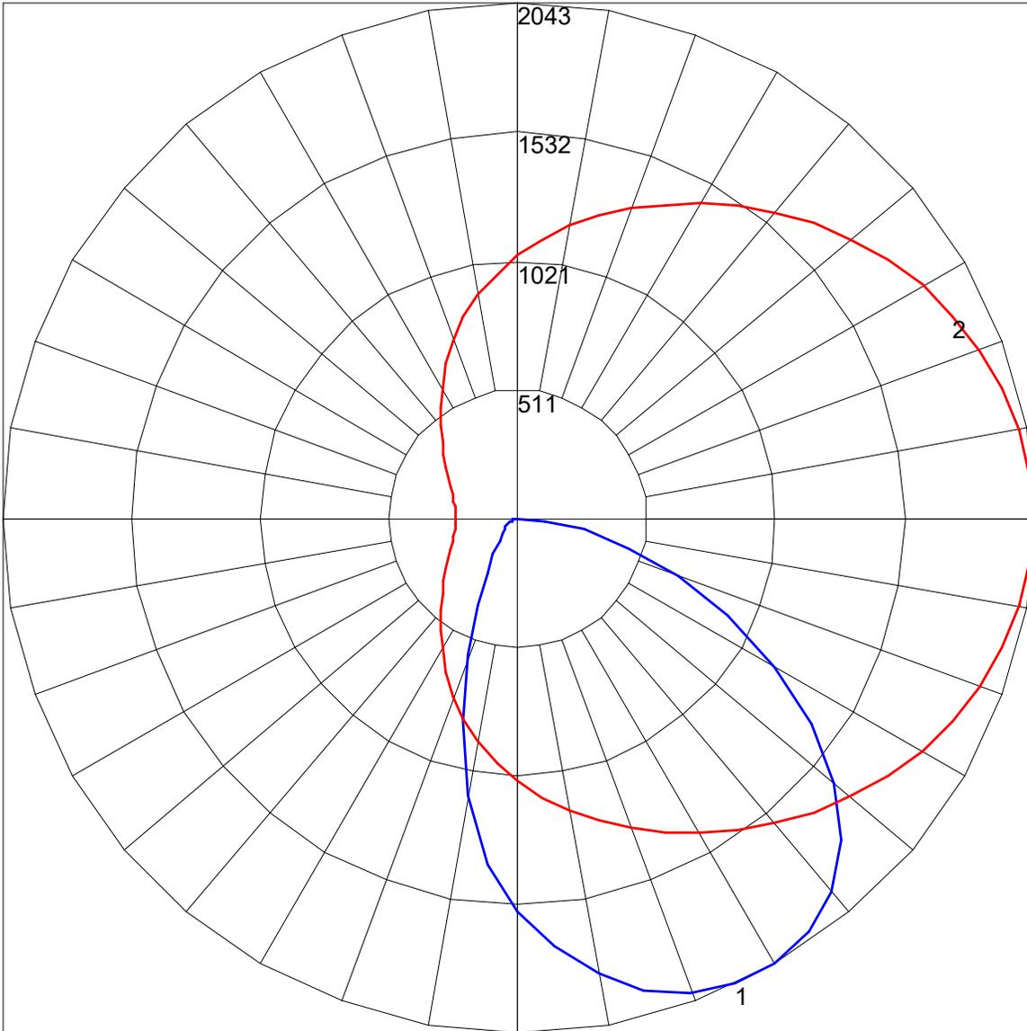
Maximum Candela = 2042.568 Located At Horizontal Angle = 0, Vertical Angle = 30
