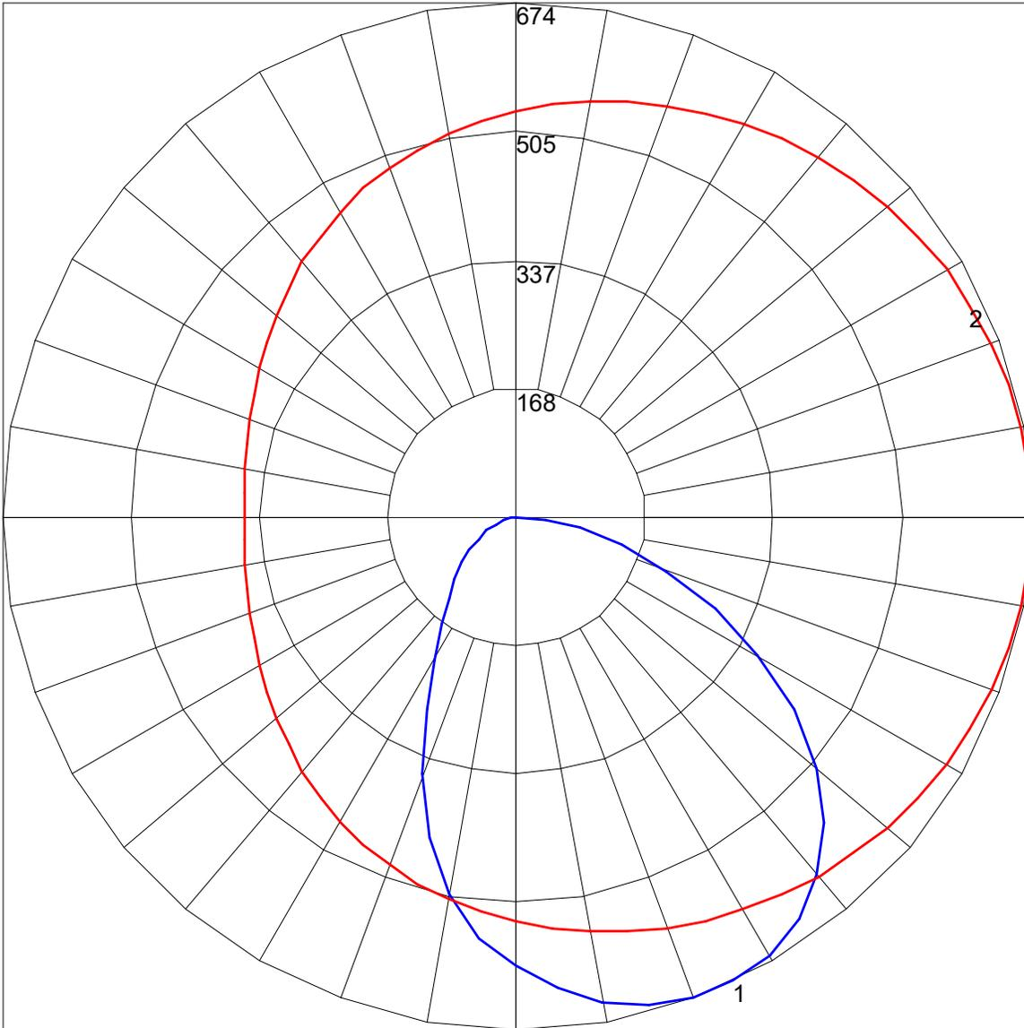
Maximum Candela = 673.96 Located At Horizontal Angle = 0, Vertical Angle = 20
