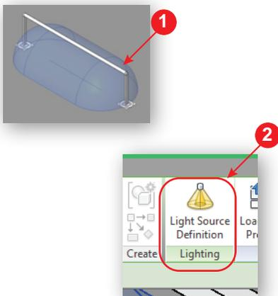
Change the light source shape to **Linear** and light distribution to **Photometric Web**.
