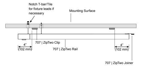
Suspended Grid Mount | 707 | ZipTwo Square 3535 | Remote Power | Suspended Ceiling Clip | Installation Guide | vodeCONNECT™ | April 2024 | Rev A • 6 of 20
