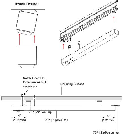
Suspended Grid Mount | 707 | ZipTwo Square 3535 | Remote Power | Suspended Ceiling Clip | Installation Guide | vodeCONNECT™ | April 2024 | Rev A • 7 of 20
