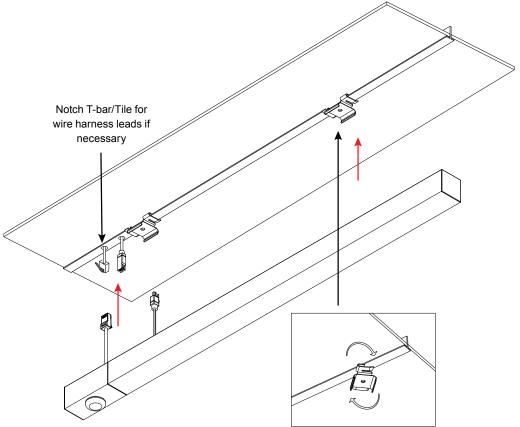
Suspended Grid Mount | 707 | ZipTwo Square 3535 | Remote Power | Suspended Ceiling Clip | Installation Guide | vodeCONNECT™ | April 2024 | Rev A • 4 of 20
